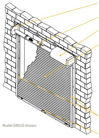
**BRACKETS** - Steel with powder coating to match curtain. Bolt to guide assembly and support counter-balance shaft curtain.
